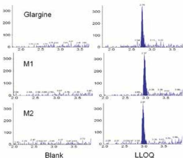
Figure 8. Chromatograms of extracted blank and LLOQ (50 pg/mL) from human plasma for insulin glargine and catabolites M1 and M2.
