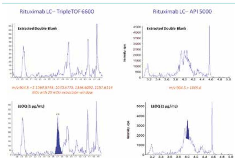
Figure 1. Comparison of the Sciex TripleTOF 6600 and Sciex API 5000 for extracted blank and LLOQ response for the Light Chain of the monoclonal antibody (mAb) Rituximab following pellet digestion.
