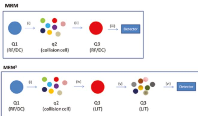
Figure 2. Comparison of events involved in the MRM and MRM<sup>3</sup> experiment on the Sciex QTrap, a hybrid quadrupole/linear ion trap.
