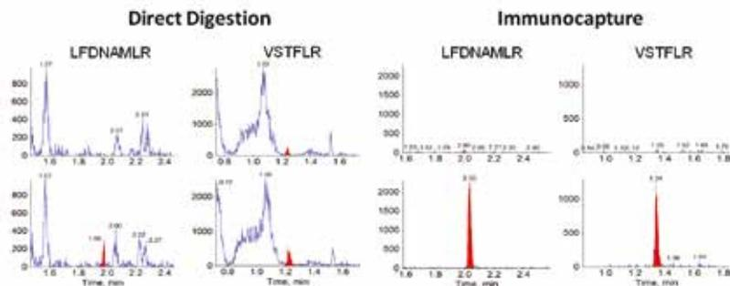
Figure 5. Blank and LLOQ (25 ng/mL) chromatograms of the two surrogate peptides used to quantitate Pegvisomant derived from rat plasma extracts using direct digestion (left) and pre-digestion anti-PEG immunocapture (right).
