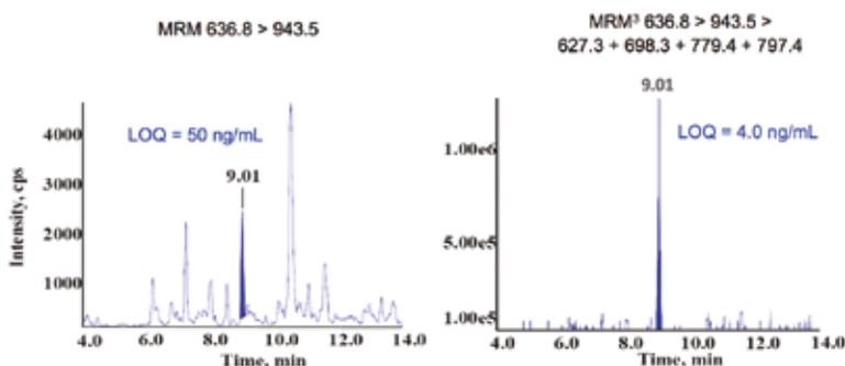
Figure 3. Reduction in background interference using MRM<sup>3</sup> in the LIT for the analysis of PSA in non-depleted human serum.
