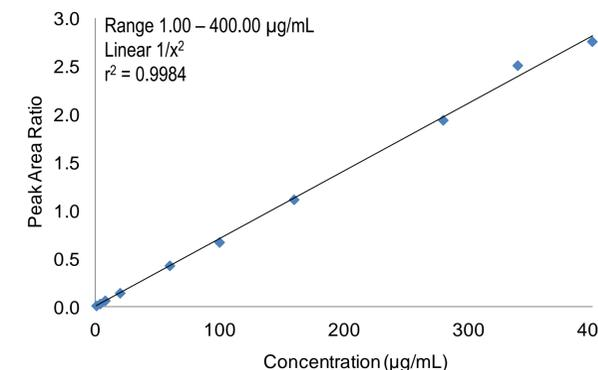
Figure 7. Calibration curve of Rituximab extracted from Mitra®
