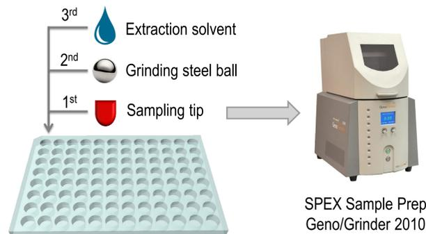
Figure 2. Impact Assisted Extraction (IAE)
